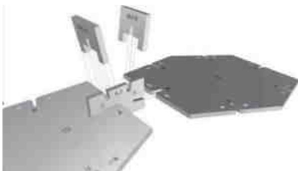
Figure 5. The digital version of the main connector and one of the locks.
