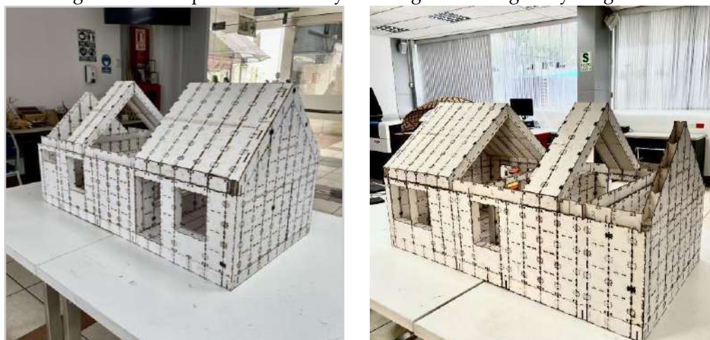
Figure 20. Physical model in 1/10 scale of the modular house.
