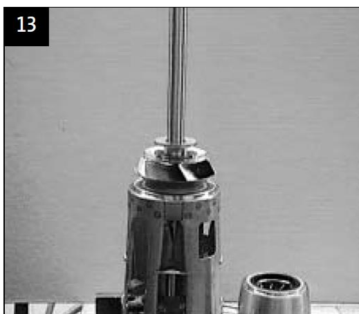
Shaft with impeller fitted in suction interconnector
