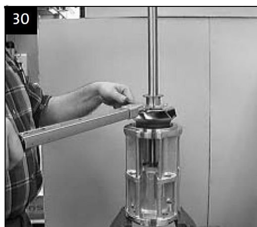
Tighten split cone nut
