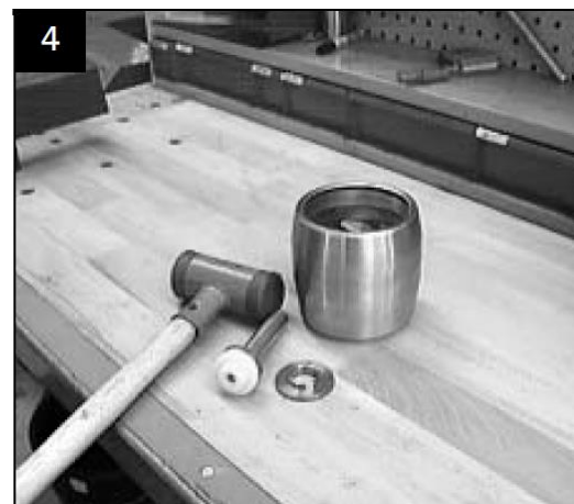
Fit stationary stop ring in chamber
