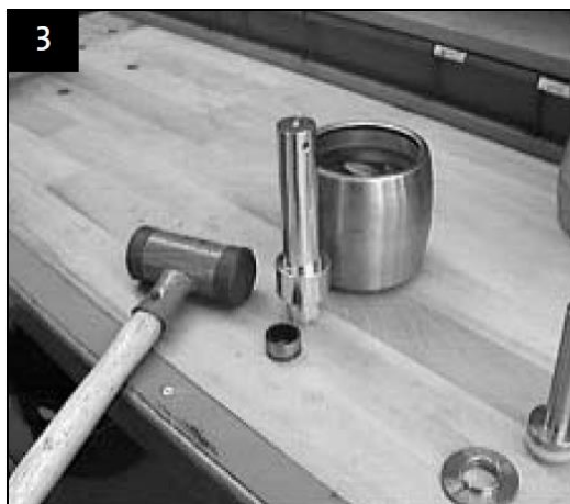
Fit lower bearing in chamber
