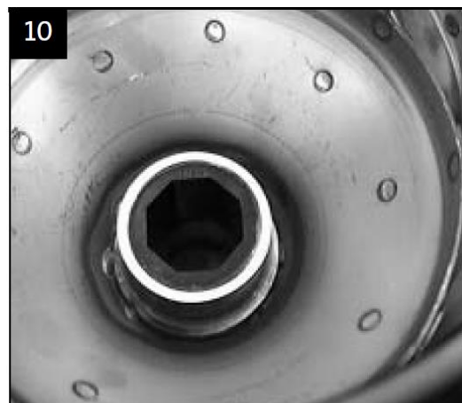
Fitted upper bearing
