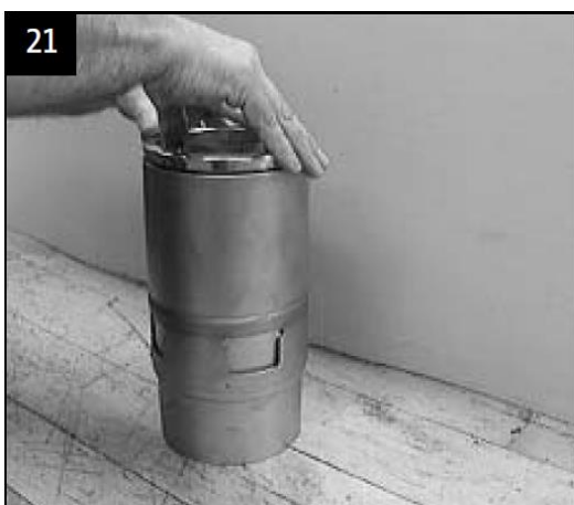
Fit retainer in valve casing
