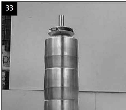
All impellers and chambers fitted
