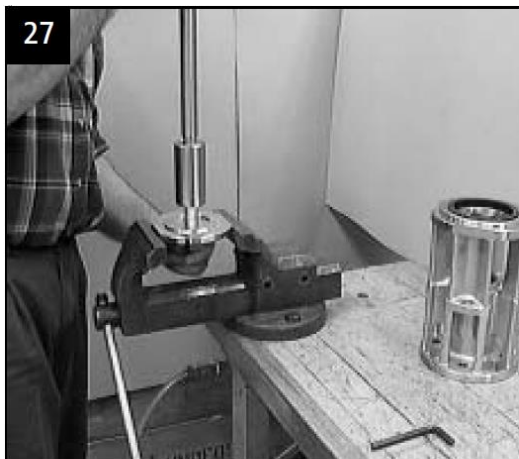
Tighten mounting plate and spacing pipe with a screw
