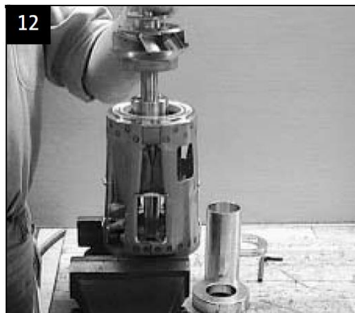
Fit shaft with impeller in suction interconnector
