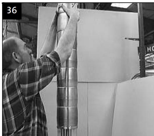
Fit valve casing
