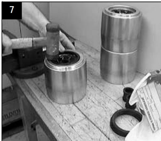
Fit neck ring in chamber
