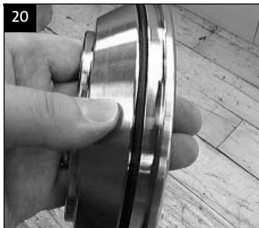
Check that O-ring is placed correctly on valve seat retainer
