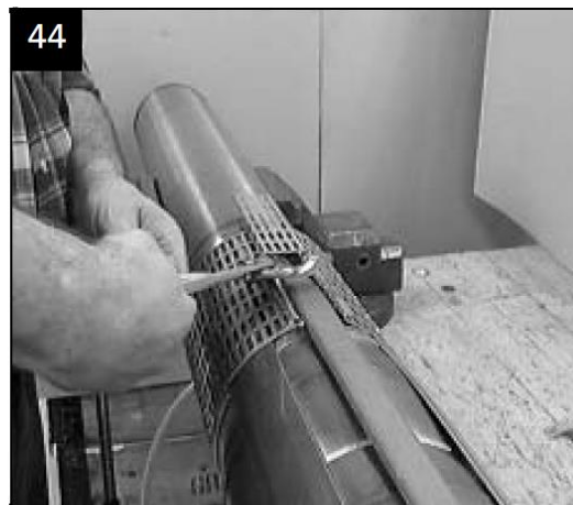
Fit lock for strainer and secure
