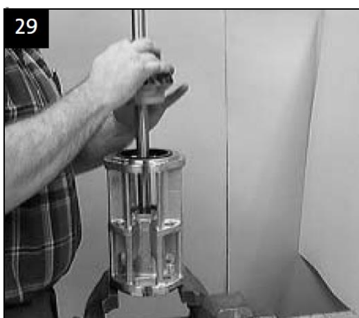
Fit first impeller including stop ring
