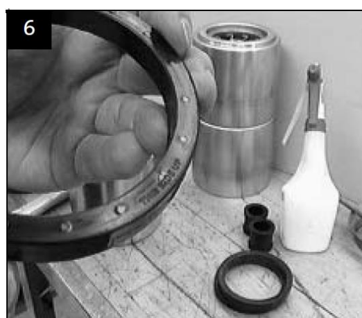
'THIS SIDE UP' must point upwards
