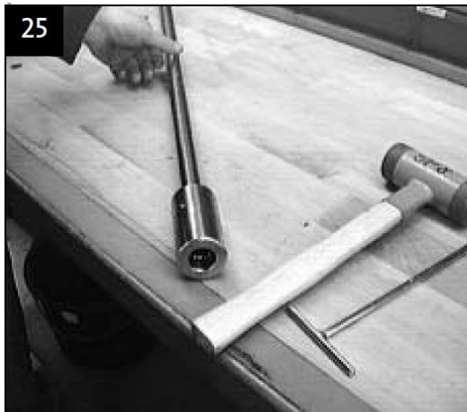
Fit coupling on pump shaft
