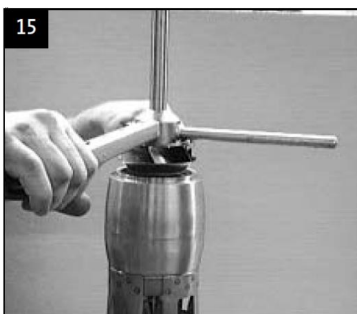
Fit next impeller
