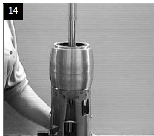
Fit bottom chamber with spacing washer for stop ring
