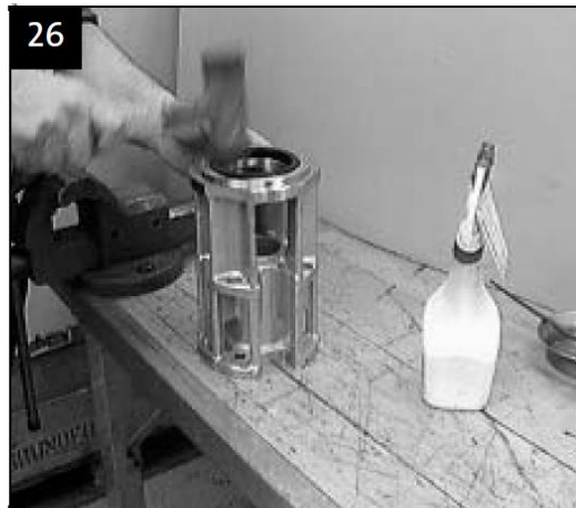
Fit neck ring on suction interconnector
