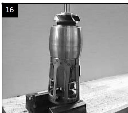
Bottom chamber and impeller fitted. Continued on page 18.
