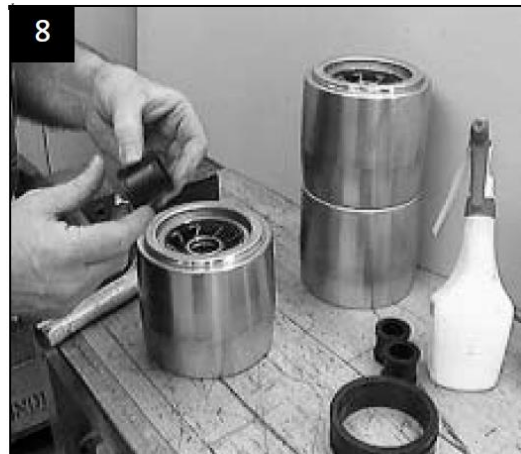
Fit rubber bearing in chamber
