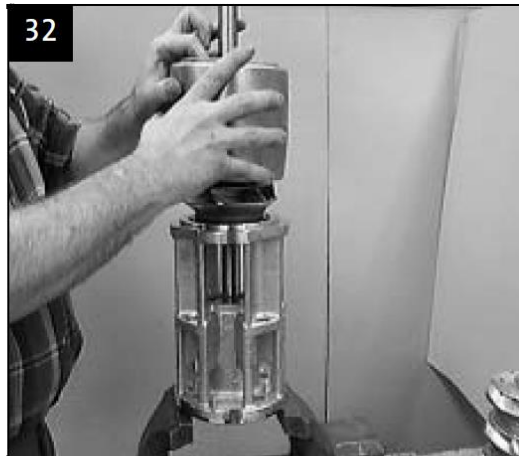
Fit bottom intermediate chamber stop ring
