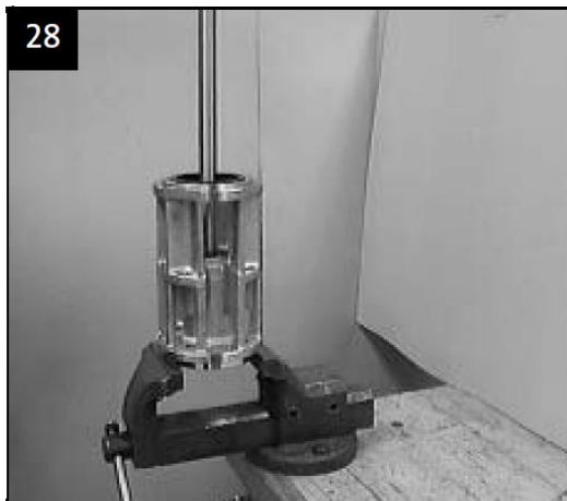
Fit suction interconnector on mounting plate
