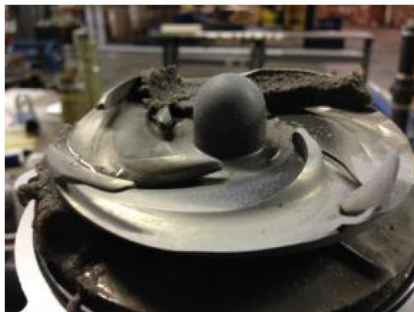
Eroded Pump Impeller
