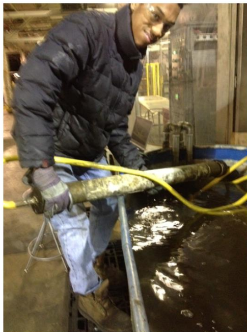
Pictured above: Pipe removal after impulse test is complete.
