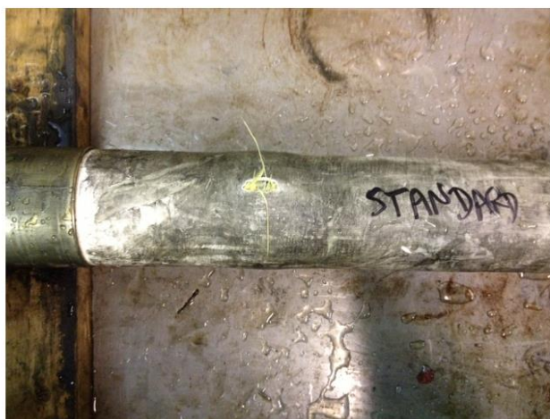
Pictured above: Standard Pipe after break which occurred at 1984.2 psi
