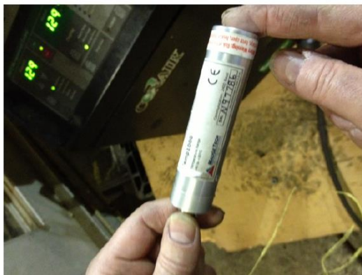
Pictured above: photo of the temperature logger used to record the temperature of the water during testing.
