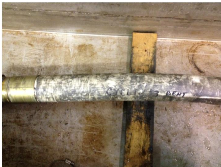
Pictured above: Cyclic Sample #3 which has a slight bend.
