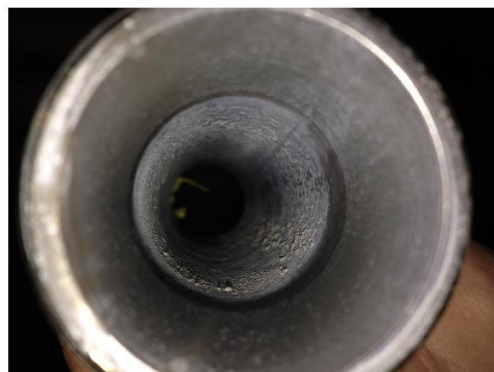
Eroded Coupling after Testing
