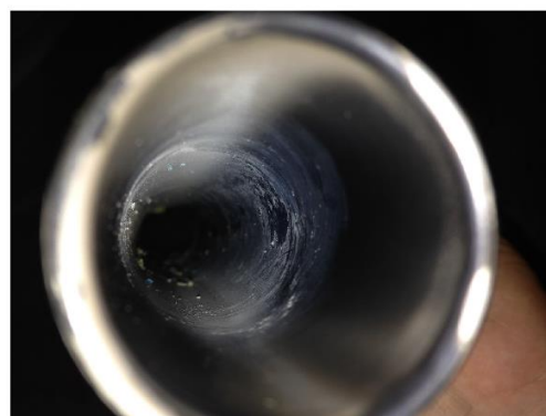
Fortron Coated Coupling after Testing Slight Erosion
