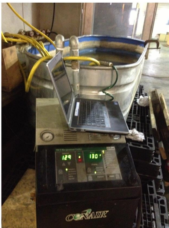
Pictured above: Tank assembly where impulse testing is performed. The tank is kept at a constant temperature.
