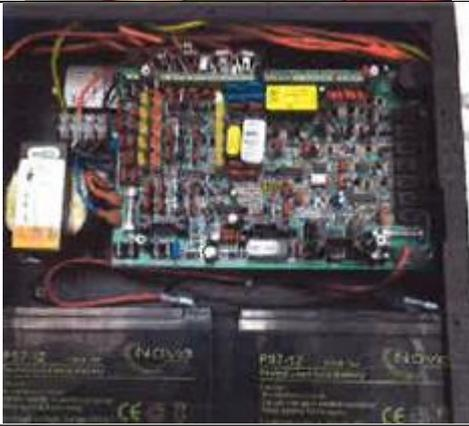
A photograph showing the interior of a fire alarm control panel. The panel is black and contains a complex array of electronic components, including a printed circuit board (PCB) with numerous integrated circuits, resistors, and capacitors. Wires are connected to the board. Two large black batteries are visible at the bottom of the panel. |
