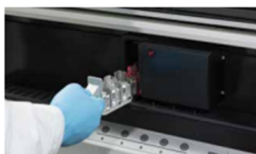
Onboard barcode reader allows real-time reagent management.
